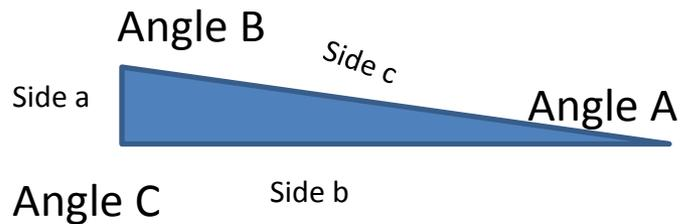
$$\text{Sine of Angle A} = \frac{\text{Length of side a}}{\text{Length of side c}}$$
